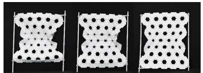
FIGURE 16: Auxetic surface tessellated by kirigami cells expands when it gets pulled down and stretched instead of shrinking.
