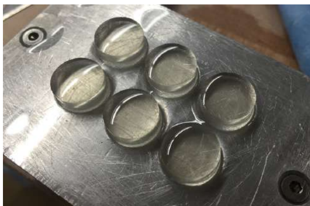
Figure 6 Ember 3D printer print plate shown with six disks to act as positives for the mould making process. Resolution and finish quality may be noted here (see online version for colours)
