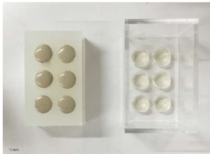
Figure 8 Positive formwork created from 3D printed disks and acrylic glass box (right) with silicone rubber mould and slip cast disks shown in liquid state (left) (see online version for colours)
