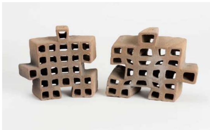
Figure 1 PolyBrick 1.0 in greenware stage after being excavated from the 3D printer and cleaned (see online version for colours)
