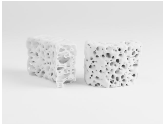
Figure 2 PolyBrick 2.0 is generated with the rules, principles and behaviour of human bone formation
