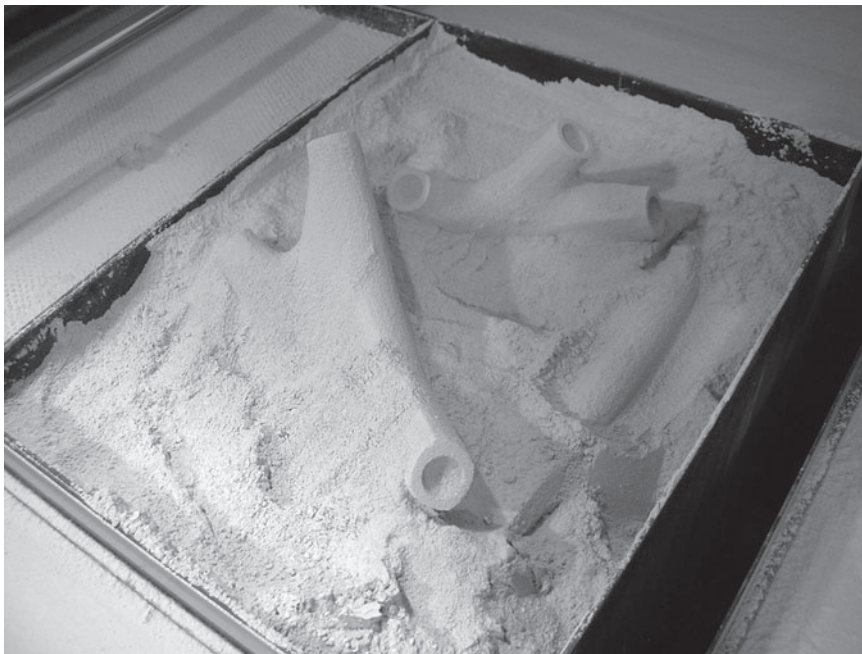
Figure 3. Three-dimensional (3D)-printed clay components for the project Ground Substance ready to be excavated from our ZCorp 510 printing bed. Figure originally featured as part of ACADIA 2010. 6
