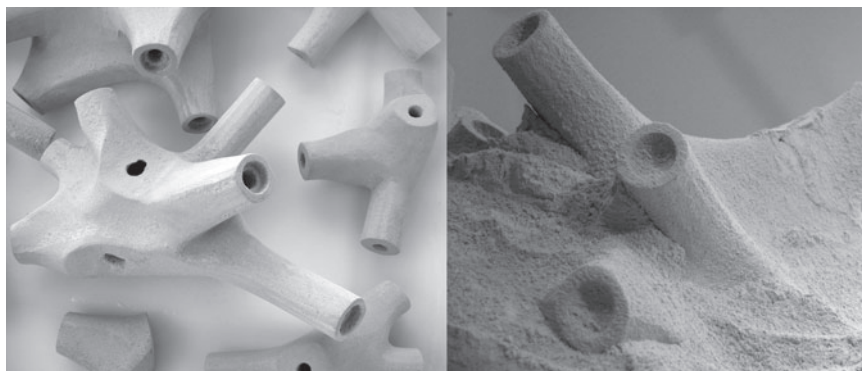
Figure 4. The greenware stage (prefiring). Excavated and cleaned 3D-printed clay parts. Figure originally featured as part of ACADIA 2010. 6
