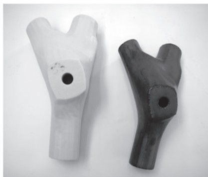
Figure 5. Initial set of prototype parts. During the initial firing, the clay body shrunk by approximately 15%. The same 3D-printed part was printed in standard starch powder (left) and in clay, then bisque fired, glazed, and glaze fired (right). Figure originally featured as part of ACADIA 2010. 6
