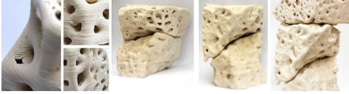
Figure 7. PDM based fabrication results of \frac{1}{4} scale and full scale PolyBrick modules demonstrating the successful utilization of proposed geometry generation and adaptation algorithms contained in the PolyBrick plug-in.
