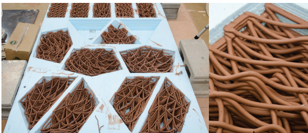
14 (Left) Component geometry and local patterning tests in dark brown stoneware. (Right) Detail of unique material behavior in clay.
