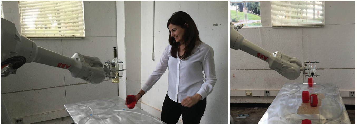
7 Dynamic wine pouring with object detection, shortest path calculation between objects and immediate tool path generation for pouring. This test highlights two levels of feedback: 1. Through a user moving their glass in space and 2. Between multiple glasses in shifting locations on a table. The tool path adjusts accordingly in real time for both cases.
