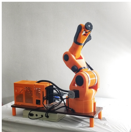
Figure 1. PICA, a Designer Oriented Low-Cost Personal Robotic Fabrication Platform.
